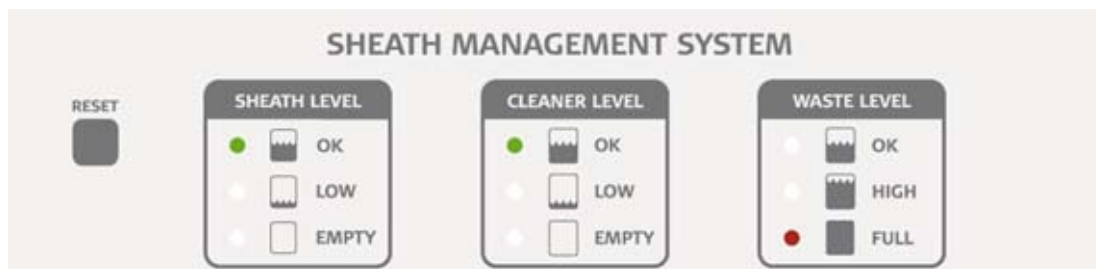
Figure 7.8 SMS Waste Full
