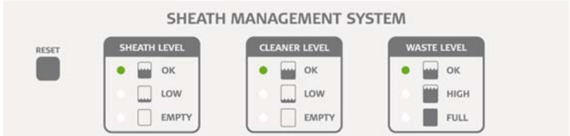
Figure 7.4 SMS Fluid Levels are Suitable for Operation
