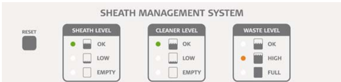
Figure 7.6 SMS High Waste Level
